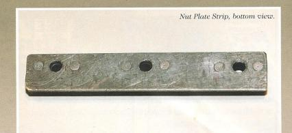
screw grip from bottoming out. Because I used nut plates, I couldn't use washers, and it was much easier to use full thread screws of adequate length. This did not present a problem, however, since the screws themselves are not used specifically to line up the structures through which they pass, but rather to hold the hinge in place by sandwiching it between two layers of aluminum sheet. Thus there is no need to have a grip on the screws.
